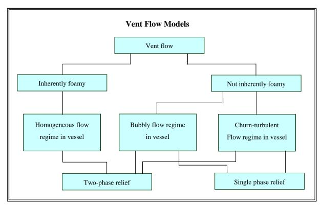
The vessel and vent flow models should be established experimentally. The following assumptions are considered conservative (safe):
