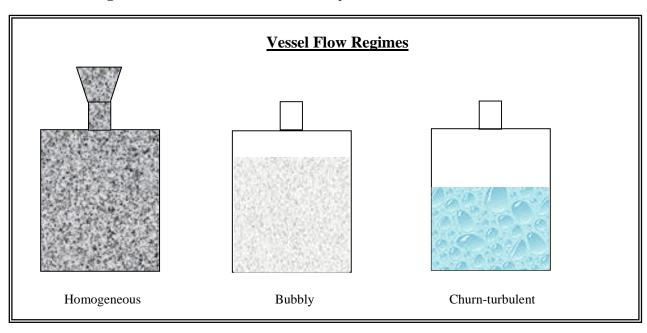
Level swell, depending on reactor level, results in venting of a two-phase mixture typical of gassy and hybrid systems.
