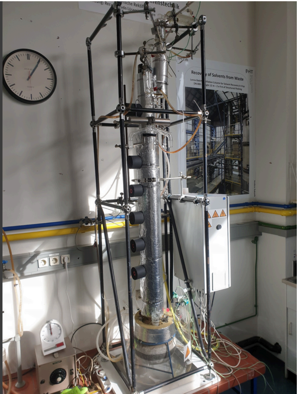
Figure 2: Batch distillation plant in the TPT lab of the Berlin University of Applied Science.
