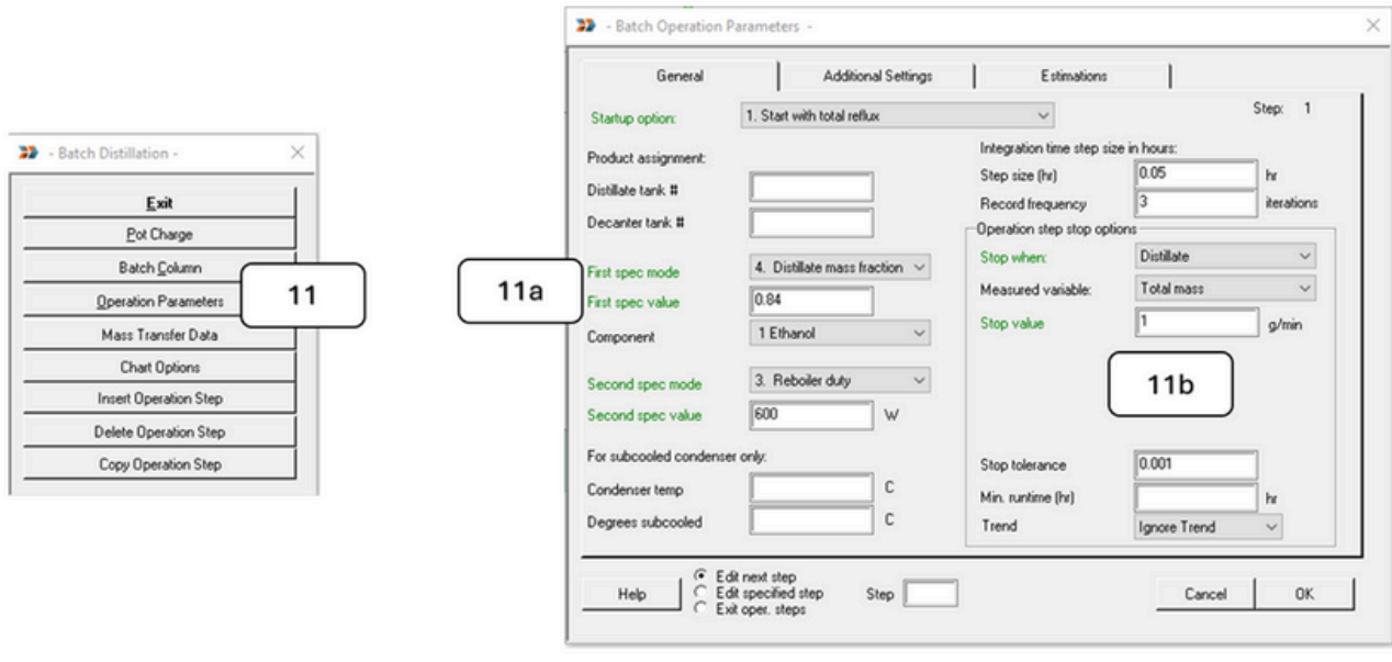
Figure 12: First Feasibility Check - Steps 11a and 11b.
