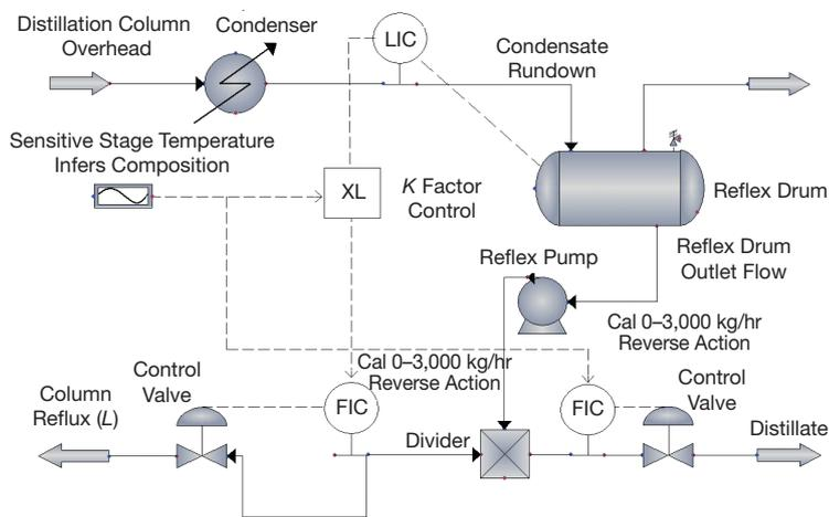
▲ **Figure 10.** The composition of the overheads from this distillation column are controlled by a feed-forward control scheme in which output of the level controller and the distillate flowrate determine the reflux flowrate.
