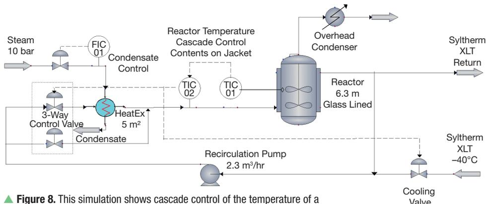
▲ **Figure 8.** This simulation shows cascade control of the temperature of a stirred-tank batch reactor.
