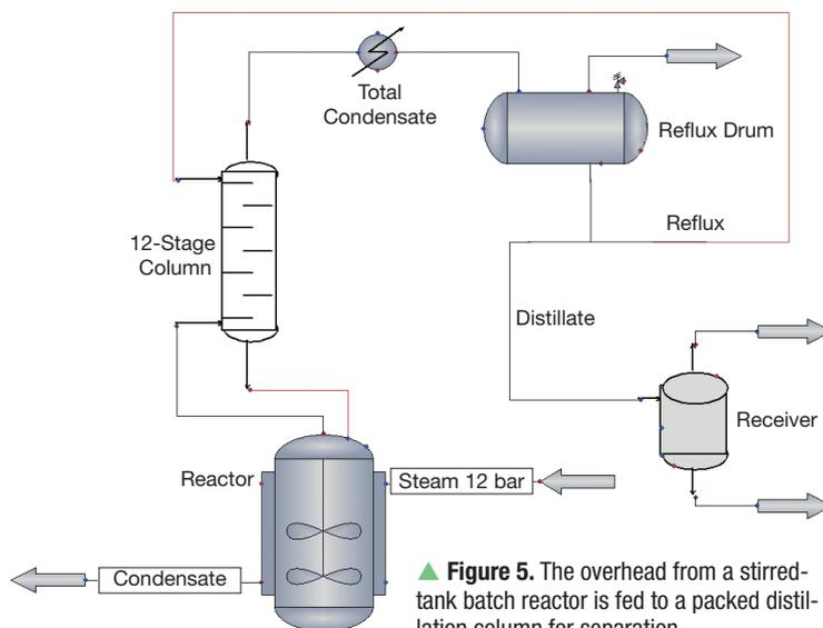
▲ **Figure 5.** The overhead from a stirred-tank batch reactor is fed to a packed distillation column for separation.
