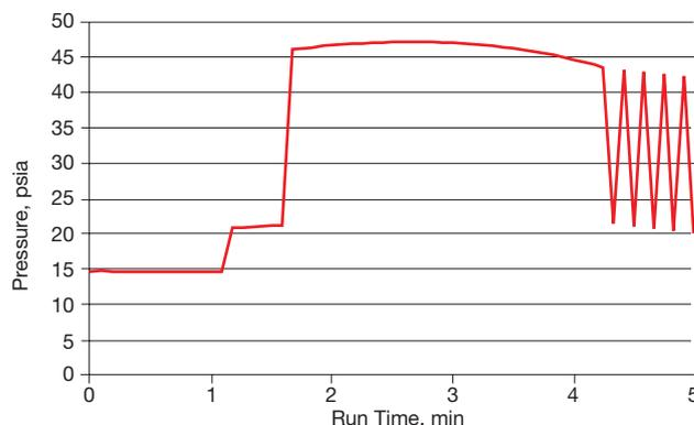
▲ **Figure 4.** This plot depicts the pressure at the exit of the relief device on Vessel 1 in Figure 3 during emergency relief of the two tanks at about 1.2 min and 1.7 min.
