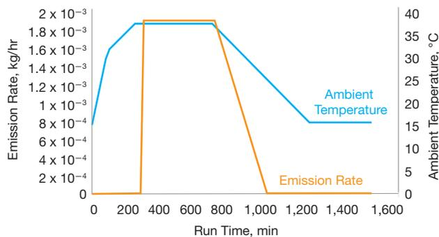
▲ **Figure 1.** A dynamic simulation can predict emissions from storage tanks due to ambient temperature changes, referred to as diurnal breathing.
