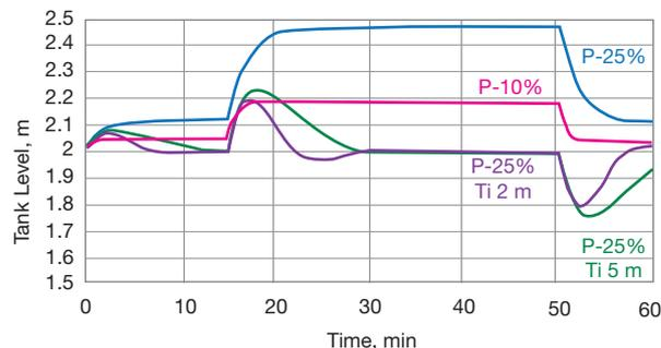
▲ **Figure 7.** The flowrate to a tank is variable and the flow from the tank is controlled by level control. The controller's tank level setpoint is 2 m, and the inlet flow increases at 15 min and decreases at 50 min. With only proportional control (blue and pink lines), there is no error control and the tank level does not reach 2 m. When proportional-integral control is implemented (green and purple), the error is eliminated.
