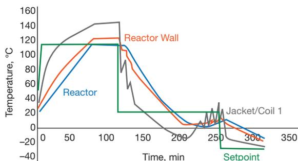
▲ **Figure 9.** The controller setpoint reaches a maximum (110°C) during heat-up and reaction, and then decreases for two periods of cooling. The cascade control scheme effectively maintains the reactor temperature, which never overshoots the maximum setpoint temperature.
