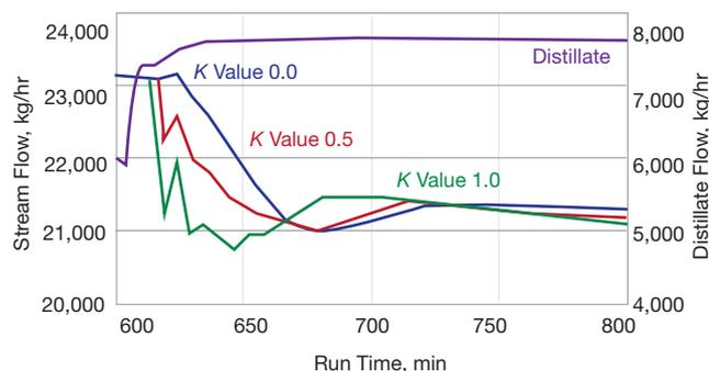
▲ **Figure 11.** When the  $K$  value is 0, the reflux flow is determined only by the level controller. It experiences a significant lag and slow rate of change. The larger the  $K$  value, the larger the effect changes in the distillate flow have on the reflux flow.
