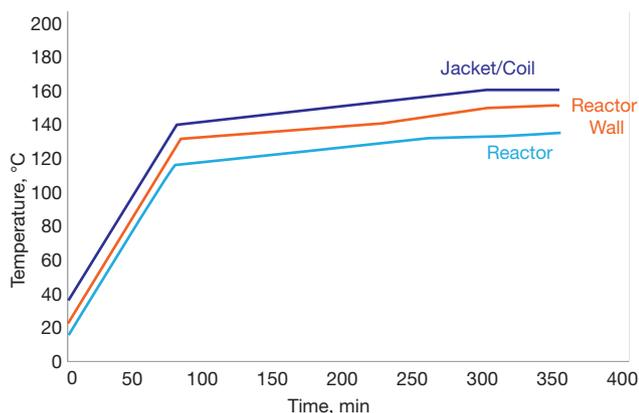
▲ **Figure 6.** The temperature difference driving force is the difference between the utility stream maximum temperature and the temperature of the vessel contents. In this case it is approximately 20°C, which enables sufficient heat transfer to the vessel contents.
