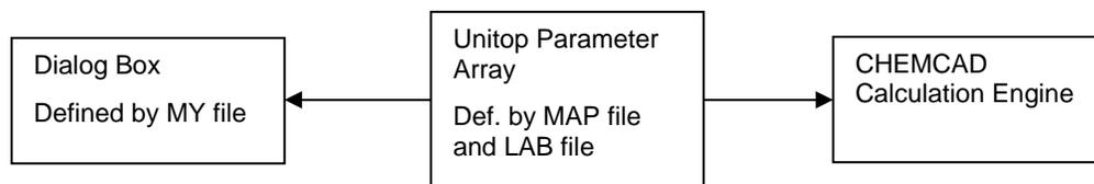
As you can see data transfer goes in both directions, meaning that calculated results for a unit are passed to the dialog in the same way that data is passed from the dialog into CHEMCAD. The Unitop Parameter Array performs any data conversions necessary, so that you might enter a value of 100 degrees Fahrenheit in a dialog, but the program sees a value of 559.67 degrees Rankine.
