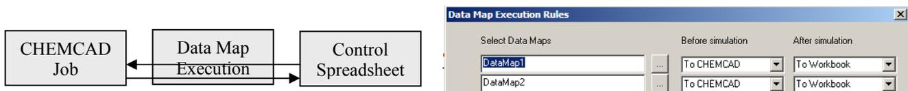
The Excel program has a control macro, located and activated from Add Ins, installed which enables the CHEMCAD model to be linked and controlled from the tool bar using the features shown.
