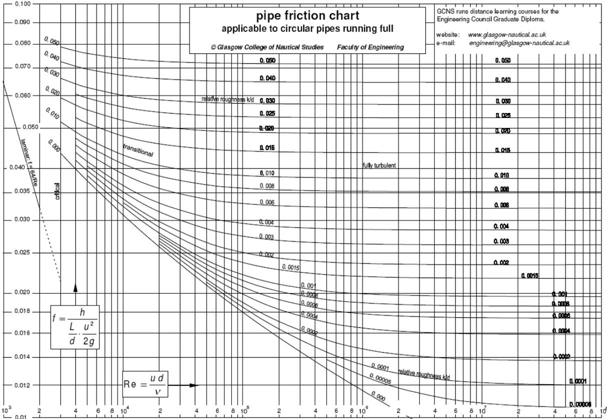
Example Friction factor for cast iron pipe  $D = 500\text{mm}$ ,  $\epsilon = 0.5 \text{ mm}$  ( $\epsilon/D = 0.001$ ) with  $Re$  of 300000 is 0.026
