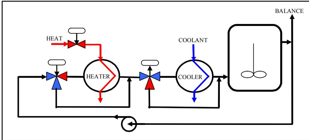
This arrangement requires an adequate recirculation flowrate determined by the reactor size and number of mixing nozzles. The jacket inlets have mixing nozzles fitted to induce a rotational flow in the jacket and enhance heat transfer. Nozzles should be fitted to induce circulation in the same direction of rotation. Inadequate flow and / or high viscosity at low temperatures will result in poor heat transfer and could result in loss of thermal stability when carrying out exothermic reactions.
