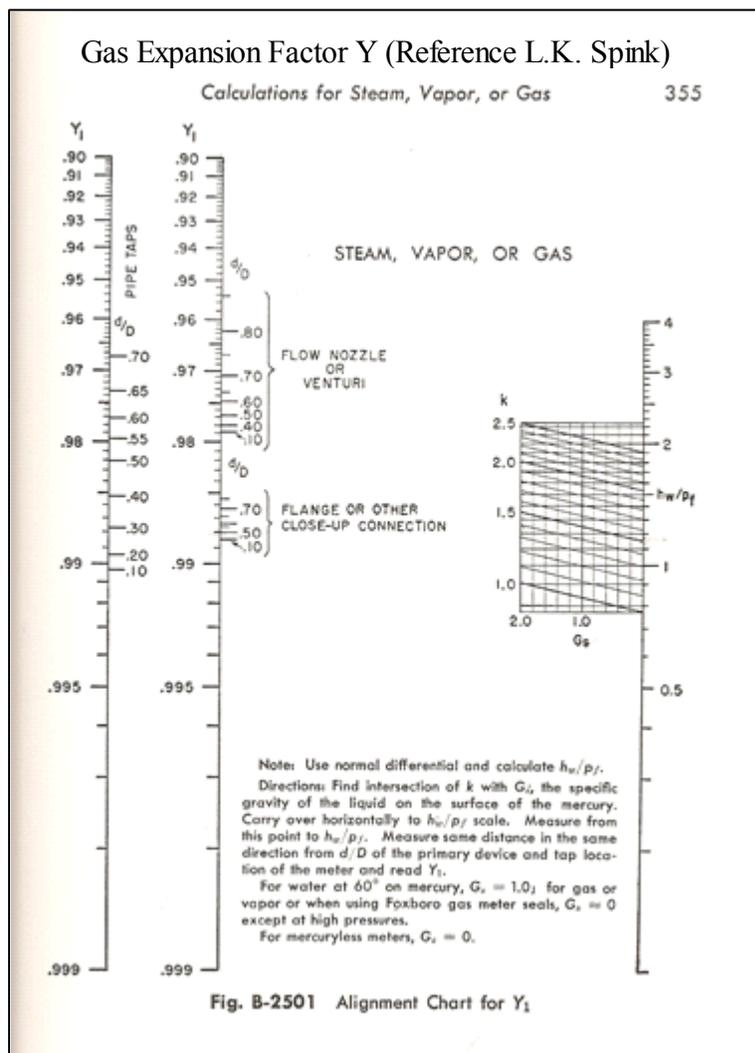
The sizing procedure is to determine an initial S and then d/D assuming F<sub>c</sub> = 1 and Y = 1. Then use alignment chart to determine Y and obtain new d/D from modified S/Y value.
