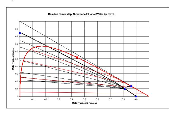
As you can see the map has distillation boundaries which cannot be crossed with conventional distillation. These boundaries partition the system into three regions. If the feed is in region one, a conventional distillation system will drive the ternary azeotrope to the top and pure water to the bottom. If the feed is in region two, the azeotrope will still go to the top but pure n-pentane will
